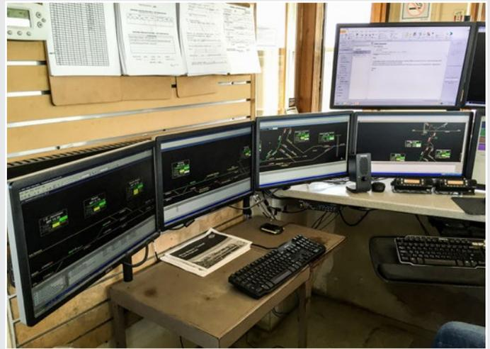
Old (left) and new dispatch systems operated together for about five weeks in the old dispatch tower in Peoria, IL, before transitioning fully to the new centralized dispatching from St Albans, VT. A 60-year-old wireline-based system was replaced with the new computer system, featuring modern, over-the-air, internet-protocol-based technology using wayside communication controllers equipped with cellular technology.
