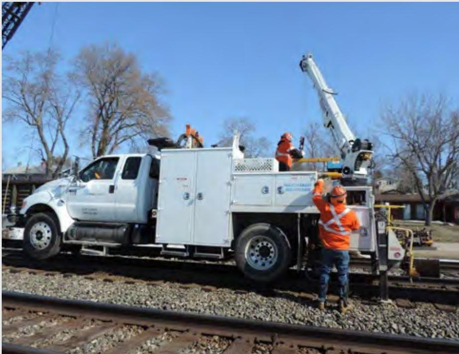
In its fleet, RailWorks Maintenance of Way has 30-plus Spec 538 welding trucks like this one, designed with convenient tool placement, customized cargo holding areas and other features specially for welding operations. The Maintenance of Way group performs extensive welding services for Class 1 railroads.
