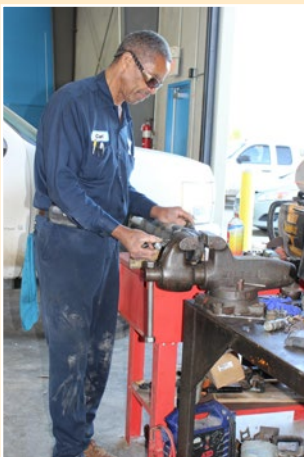
Carl Preston is one of three mechanics on site at RailWorks Track Systems' South Region hub office, located in Deer Park, TX. Carl typically works on backhoes, loaders and hydraulic tools, among others. Here, he repairs a hydraulic thumb cylinder for a backhoe that is part of Deer Park's 300-vehicle fleet.
